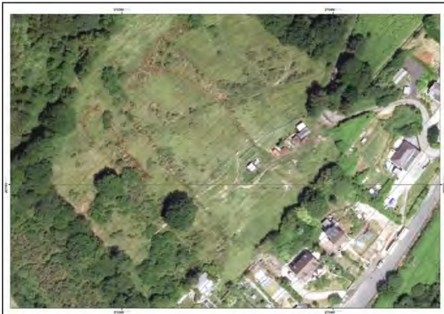
Insert 6: Enlargement of 2013 Orthophotography showing possible landslides identified in the area of "shallow slips" recorded on the geological map
