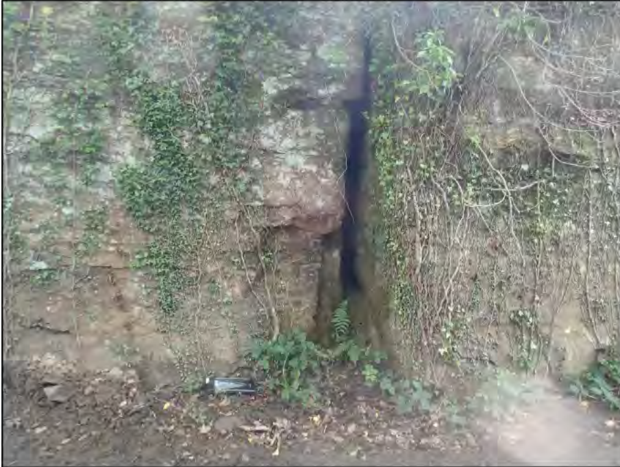
Plate 5: Bedding dipping from left to right (20/185) the rock face is formed by joint set 84/274 and the dilated joint set is formed by 74/018.
