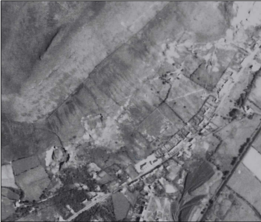
Figure 7: Extract of the 1945 Aerial photograph showing high reflectance associated with adits working the Upper Pinchin coal seam
