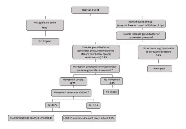
Using the probabilities assigned in the event tree, for a 1 in 100 year rainfall event (which is equivalent to 0.01), it suggests that the estimated annual probability of a landslide hitting the school is 0.0019, or 1.9x10<sup>-3</sup>.
