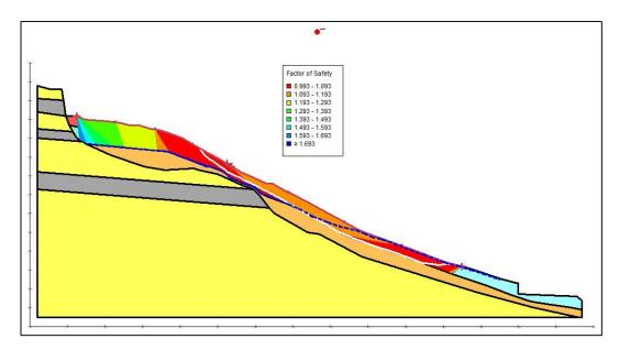
**Insert 16**: Contoured failure planes in Quarry Spoil Tip using Upper Range Parameters and groundwater at the tip base – DA1 C2.
