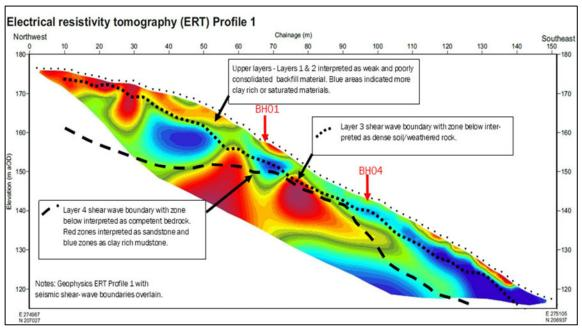
**Insert 9**: Summary of geophysical data (ERT and Seismic data) interpolated from Terradat report (2019). Full report displayed in Appendix K.
