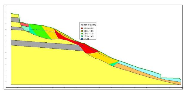
Insert 11: Contoured failure planes in Quarry Spoil Tip using Reasonable Case Parameters.
