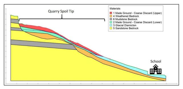
Insert 10: SlopeW digital Ground Model
